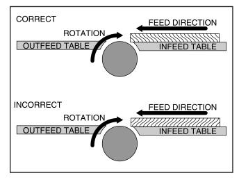
**Figure 19.** Correct and incorrect grain alignment to cutterhead.
